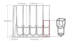
Each microwell is designed to fit the magnetic tips of all KingFisher™ purification systems using magnetic separation technologies.
