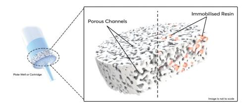
Traditional loose-filled methods for chromatography applications is often associated with poor and inconsistent flow rates. This is largely due to the inherent problems with packing of loose particles (over-compression, under-compression and voiding) in wells and columns. Packing inconsistencies can impact not only the effectiveness of sample preparation, but the reproducibility and reliability of results obtained.
