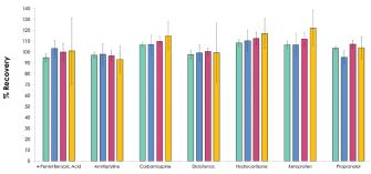
The Microlute<sup>™</sup> hybrid technology is designed to capture phospholipids and allow small molecules (analytes) to smoothly pass through unaffected. Get greater than 90% recovery with high levels of reproducibility for a wide range of acidic or neutral analytes.
