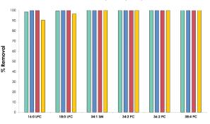
Consistent flow rates of biological fluids through the filter results in greater interactions with the active media throughout the 96-well plate, allowing precise and specific removal of all classes of phospholipids (LPC, PC, SM).
