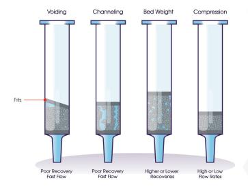
Microlute<sup>™</sup> products also eliminates the need of 'extra' flanking filters or frits for media support allowing further undisrupted flow of samples with reduced material breakthrough. Hydrophobic treatment of filters offers greater sample holdup for methods that require subsequent pull through for elution of cleaner extracts.
