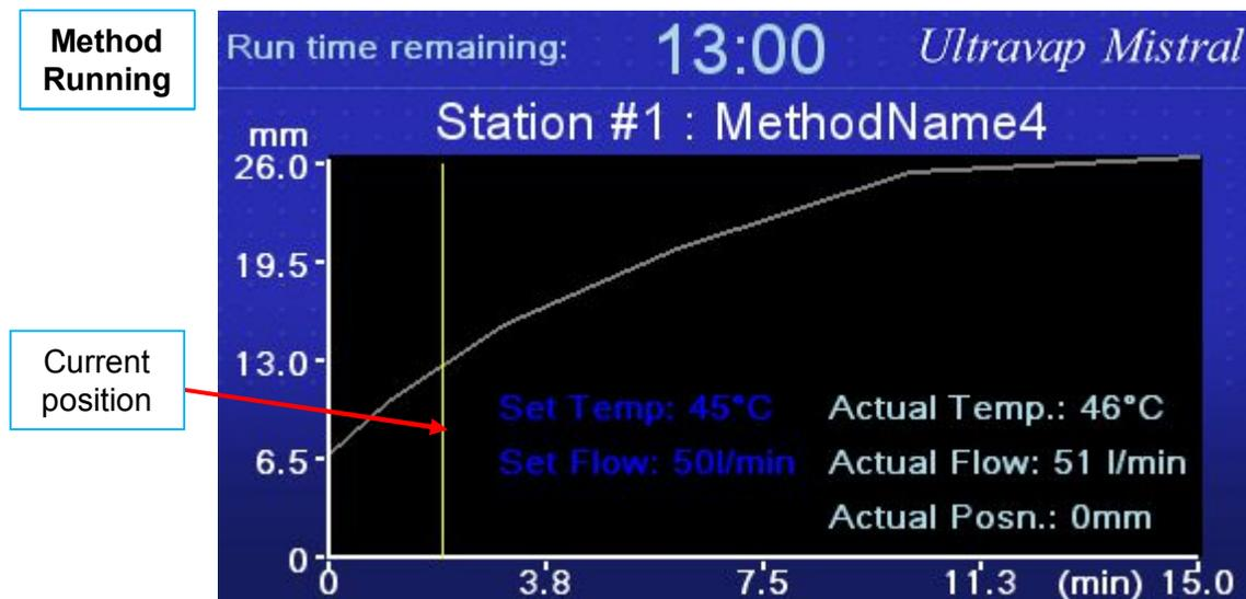
Once the instrument has finished running a method, the screen will indicate the evaporation is complete and eject the carrier to the set load position. The user can then either load a new sample and repeat same method, or select a new method to program.
