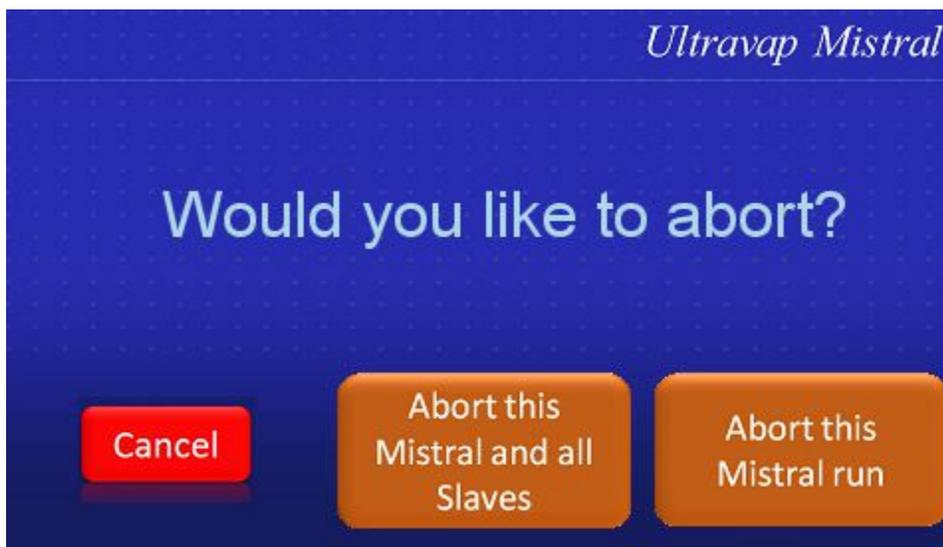
If an Ultravap Mistral needs to be stopped during a run for any reason, it can be aborted separately by pressing the screen to bring up the abort option. The user will then have the ability to abort a single Mistral run individually without affecting other connected slave units.
