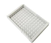
The Signum<sup>TM</sup> No Bind microplates are designed to enhance signal-to-noise ratios of highly sensitive assays by eliminating signal loss due to molecular absorbance to the surface of the plate well. Pure polystyrene is uniformly treated to prevent binding and absorbance of biomolecules to the surface of microplate wells which can result in loss or reduction in signal.
