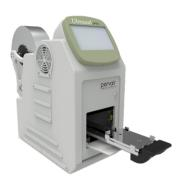
Featuring all electric operation, making it suitable for laboratory automation. The use of force sensors allows dynamic feedback during the entire sealing process to ensure homogenous sealing, all controlled through the intuitive touchscreen interface.
