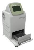
The Ultraseal™ CAP-PRO has been designed to take the strain out of applying friction sealing mats or septum sealing caps to SBS format tube racks and plates. Simply place your rack or plate with its associated friction mat or septum cap in the drawer and push it firmly shut.
