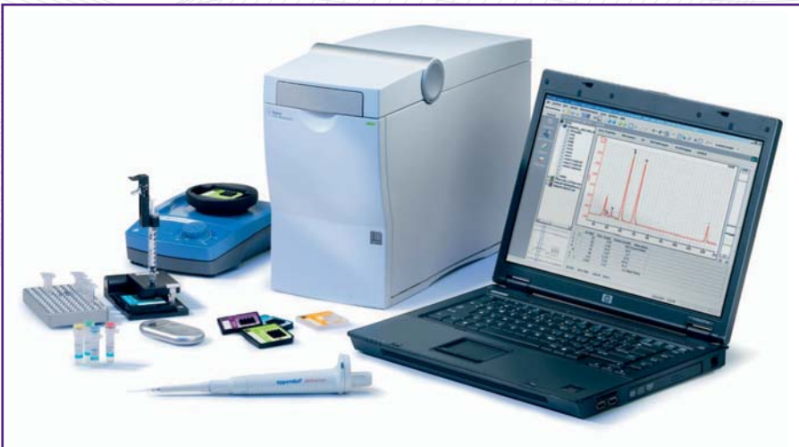
Figure 4 – The Agilent 2100 Bioanalyzer ® and high-sensitivity DNA assay components. Beside the instrument, a vortex and chip priming station are used to prepare samples for analysis. The 2100 work area software has several tabs which display data for evaluation of chip runs that can be presented as result tables, gel-like images, histograms, dot plots, or, as above, electropherograms. (Photo copyright Agilent Technologies Inc.).
